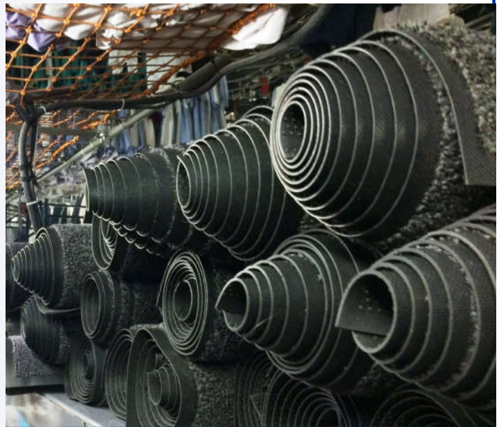
Coning Of the mats created by not starting the lead edge of the mat straight
